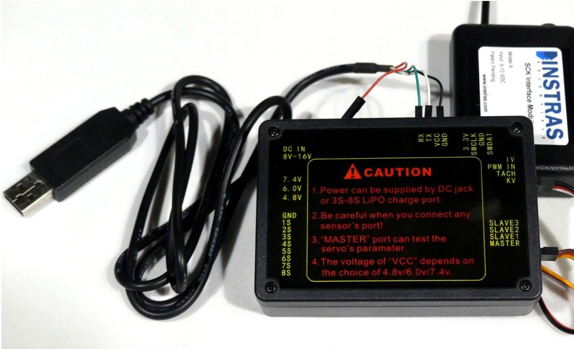
Instras PDC3 supports UART communication with 9600 baud rate, 1 stop bit and no parity bits. All commands and responses sent to or from Instras PDC are in text (ASCII) format. Every command and response ends with new line(10 in ASCII table) and carriage return(13 in ASCII table ) symbols.
